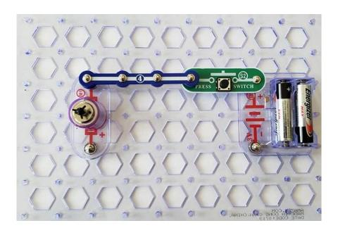
Step 7: put a 4-wire between the battery holder and the motor.
