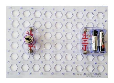
Step 3: put the motor 5 spaces away from the battery holder.
