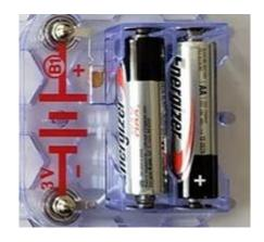
Step 1: put the batteries in the battery holder.
