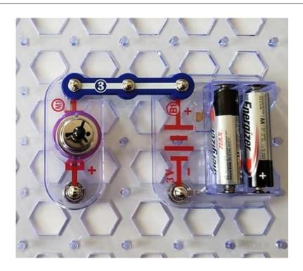
Step 4: put a 3-wire on the motor and battery holder.
