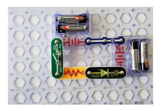
Step 7: put the green switch between the yellow resistor and the battery holder.
