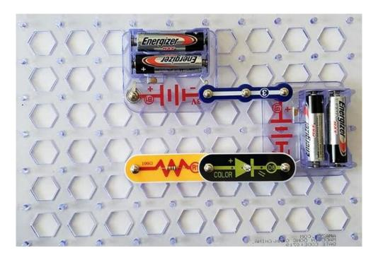
Step 6: put the black LED between the resistor and the battery holder.
