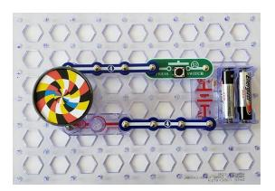
Step 12: put a spinner on the motor and push the press switch to make it spin.
